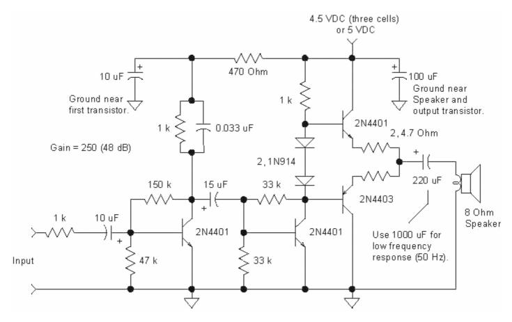
The circuit above shows a 4-transistor utility amplifier suitable for a variety of projects including receivers, intercoms, microphones, telephone pick-up coils, and general audio monitoring. The amplifier has a power isolation circuit and bandwidth limiting to reduce oscillations and "motorboating". The values are not particularly critical and modest deviations from the indicated values will not significantly degrade the performance.
