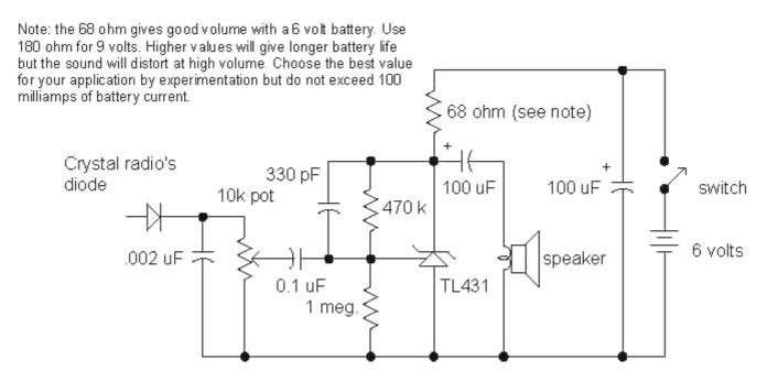
Here is the amplifier used to boost the output from a simple crystal radio. The volume control is at the bottom left and the other components are on the terminal strip at the bottom of the picture. This is a really quick and easy audio amplifier!
