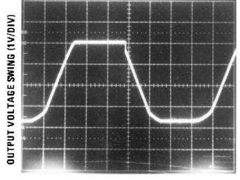
TIME (5  $\mu$ s/DIV) Figure 28. Current Limit (R<sub>L</sub> = 100 $\Omega$ )
