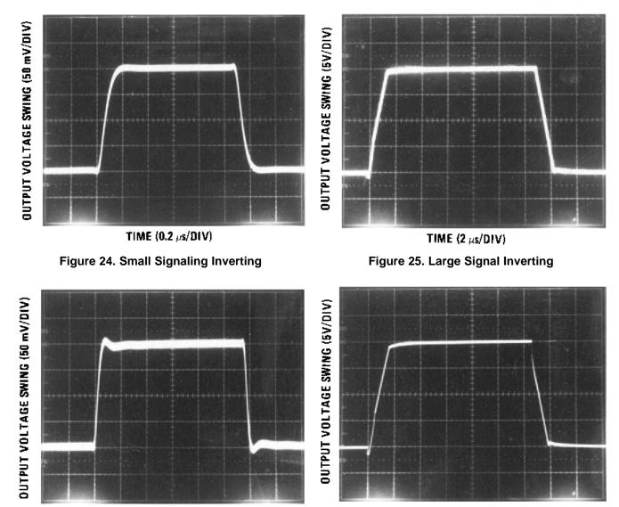
TIME (0.2 μs/DIV) Figure 26. Small Signal Non-Inverting
