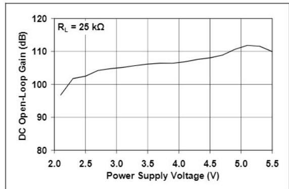
**FIGURE 2-18:** DC Open-Loop Gain vs. Supply Voltage.
