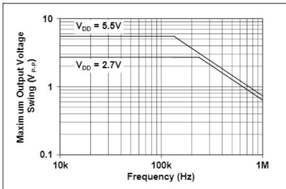
**FIGURE 2-21:** Maximum Output Voltage Swing vs. Frequency.
