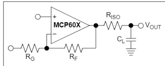
**FIGURE 4-4:** Output resistor  $R_{ISO}$  stabilizes large capacitive loads.
