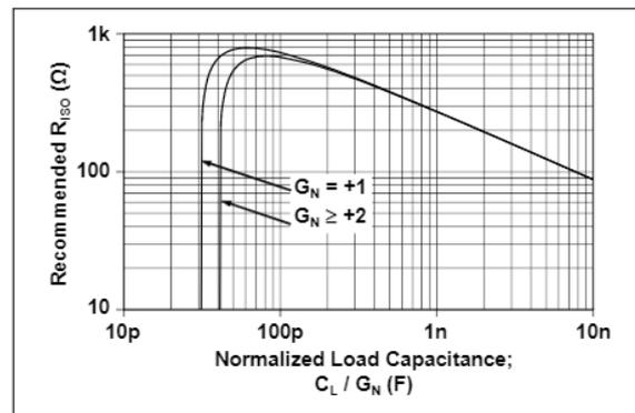
**FIGURE 4-5:** Recommended  $R_{ISO}$  values for capacitive loads.
