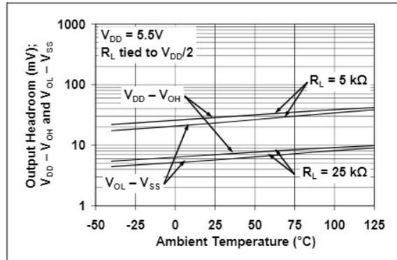
**FIGURE 2-23:** Output Voltage Headroom vs. Temperature.
