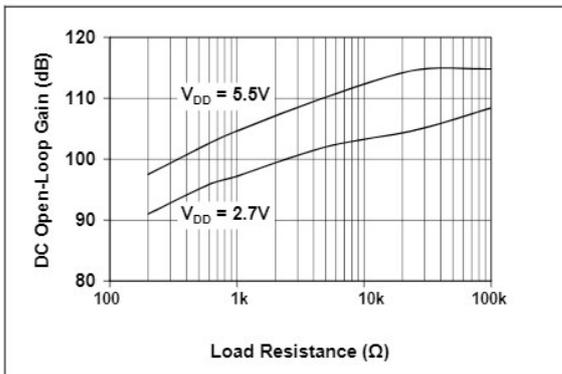
**FIGURE 2-15:** DC Open-Loop Gain vs. Load Resistance.
