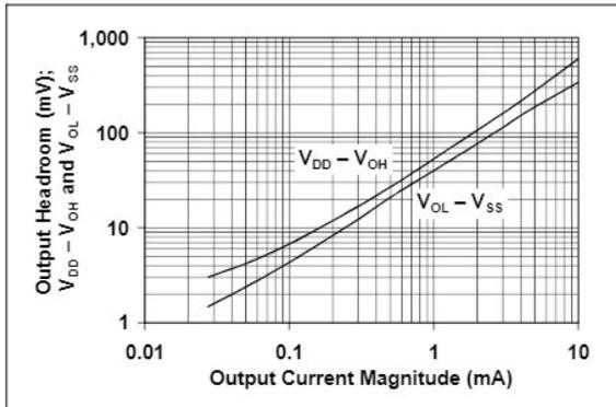
**FIGURE 2-20:** Output Voltage Headroom vs. Output Current.
