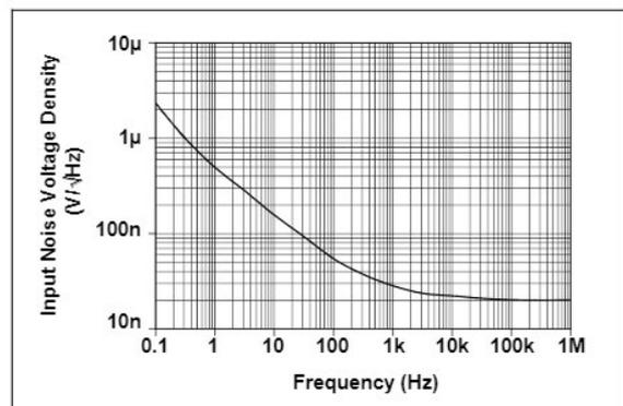
**FIGURE 2-6:** Input Noise Voltage Density vs. Frequency.
