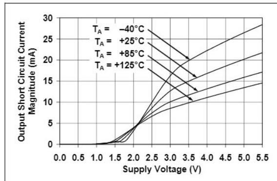
**FIGURE 2-24:** Output Short-Circuit Current vs. Supply Voltage.
