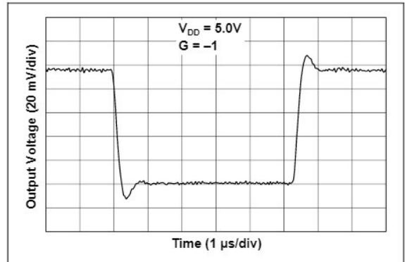
**FIGURE 2-29:** Small Signal Inverting Pulse Response.
