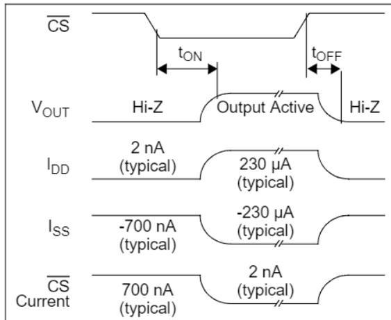
**FIGURE 1-1:** MCP603 Chip Select ( $\overline{\text{CS}}$ ) Timing Diagram.
