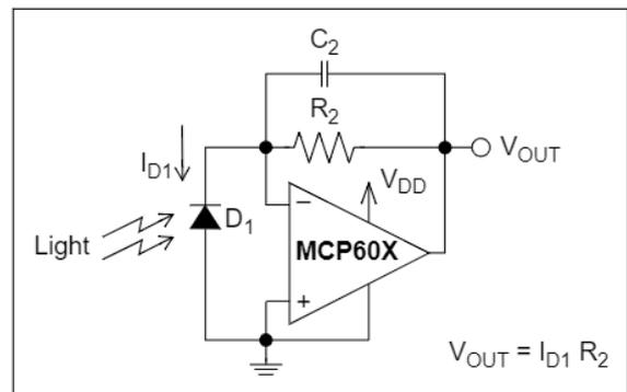
**FIGURE 4-12:** Photovoltaic Mode Detector.
