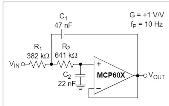
FIGURE 4-8: Second-Order, Low-Pass Sallen-Key Filter.
