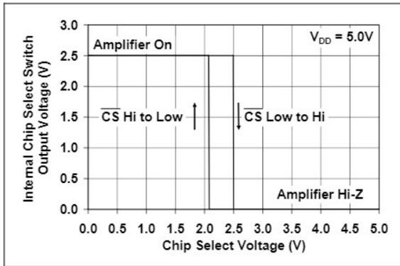
**FIGURE 2-32:** Hysteresis of Chip Select's Internal Switch.
