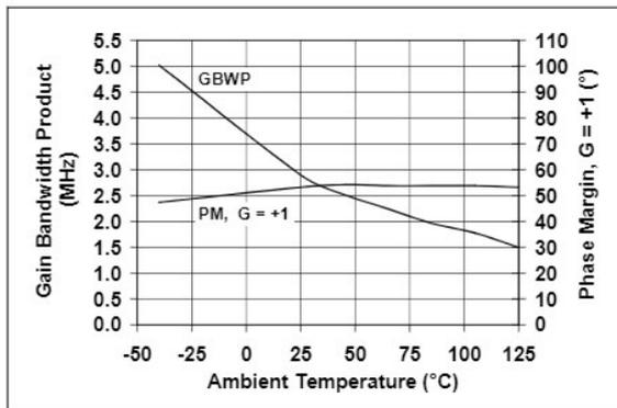
**FIGURE 2-3:** Gain Bandwidth Product, Phase Margin vs. Temperature.
